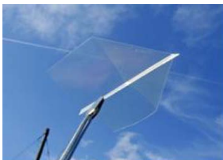
Fig. 18 The 100% cellulose nanofibre sheet is as foldable as traditional paper. Reproduction of image from [199] with permission from Wiley (© Wiley 2009)
