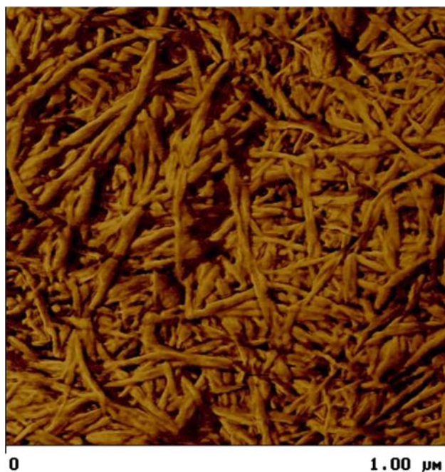
Fig. 27 AFM micrograph of cellulose nanopaper surface. The cellulose nanofibers are disintegrated from dissolving wood pulp of 95 wt% cellulose content, using an enzymatic pretreatment procedure. Image by Prof. I. Mondragon, University of Basque Country, San Sebastian, Spain
